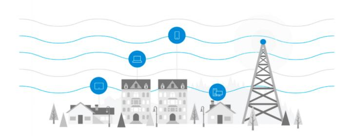
TV White Space Internet involves radio wave frequency ranges that are newly available due to the recent conversion from analog TV to digital TV. Internet signals are transmitted through frequencies that used to bring us terrestrial TV broadcasts. This particular set of frequencies can travel several miles and is affected less by blockages such as buildings. White Space Internet services are still in an exploratory stage, existing in a few test sites and experiments.
